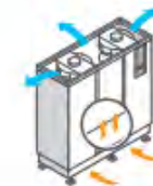
Upflow unit with suction from the base.
