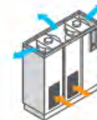
Upflow unit with suction from the front.
