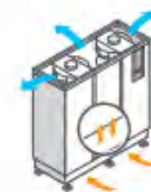
Upflow unit with suction from the base.
