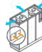
Upflow unit with suction from the rear.
