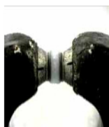
Liquid oxygen between the poles of a horseshoe magnet.
