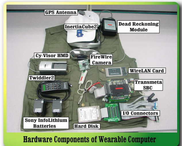
Figure 4. Detail configuration of wearable computer
