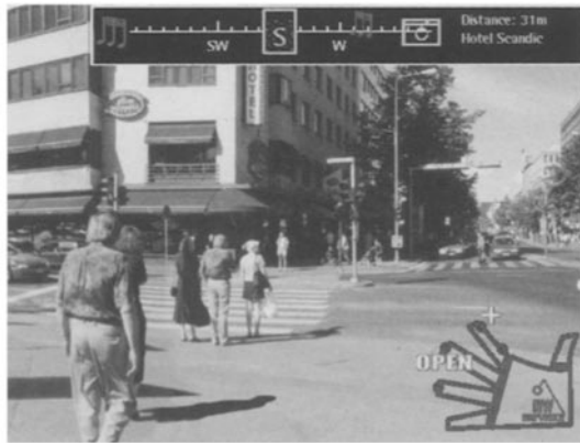
Fig. 7. ContextCompass. The user has most of the view unblocked. Virtual objects are shown on the compass. This is a synthesised image.
