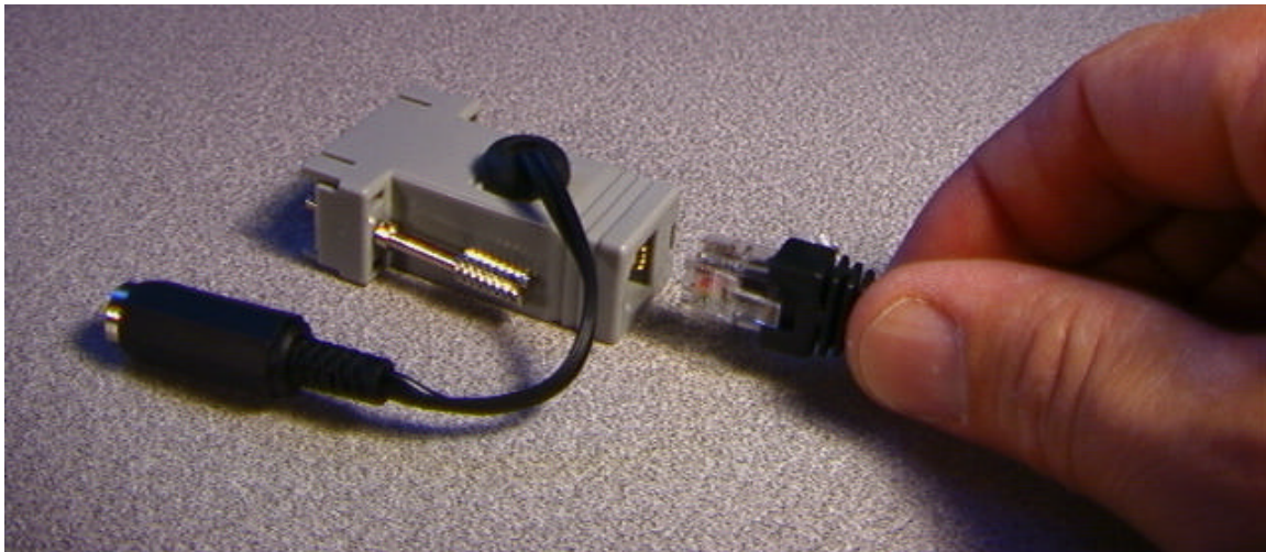
Connection of InertiaCube2 cable to serial port power dongle
