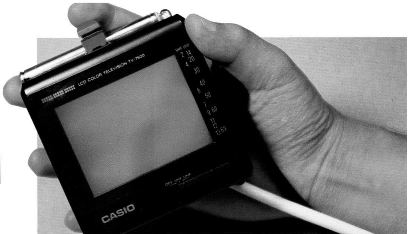
Figure 3. Palmtop unit consisting of a video display, a response button at the top of the unit and a 6D input sensor for providing x, y, and z positional information and orientation (pitch, yaw and roll)
