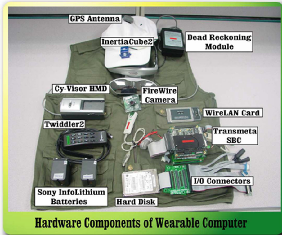
Figure 4. Detail configuration of wearable computer
