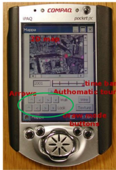
Figure 2: The User Interface developed for interacting via PDA with the Nu.M.E. VE
