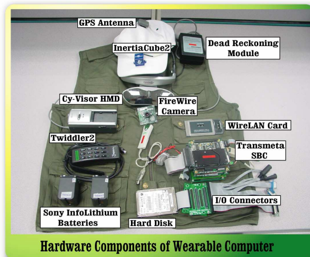
Figure 4. Detail configuration of wearable computer
