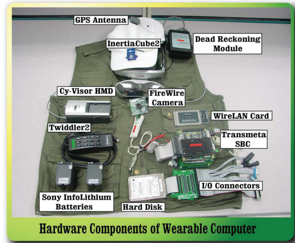
Figure 4. Detail configuration of wearable computer
