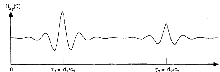
FIGURE 3.14 Cross-correlation function between source and receiver signals with two nondispersive propagation paths.
