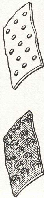
Fig. 6 : 6. 'Stabbing' of holes in main pipe wall gives superior effect in comparison with clean drilling (right).
