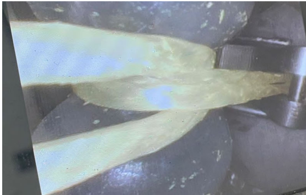
(Internal image of hemostasis valve with filaments encircling and constricting elongate member.)
