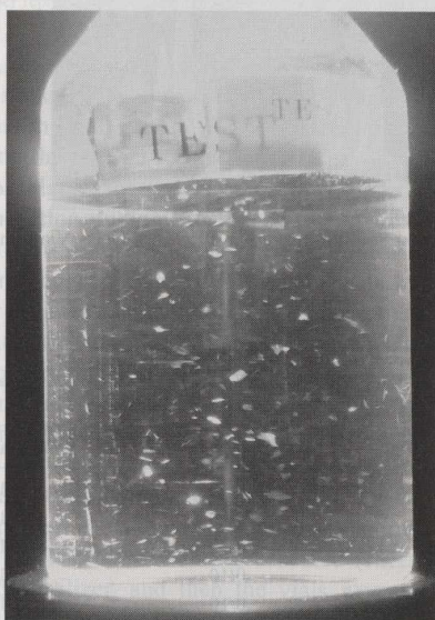
Fig. 1. The Flake-Like Particles of Phosphate Buffer Solution in a Glass Vial
