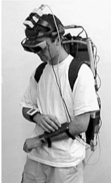
Figure 3. Users of the wearable computer see through a Sony PLM-100 transparent head-mounted display, and enter commands on a Phoenix forearm keyboard.
