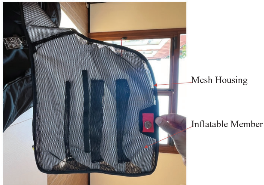
Image of Tech-Air 3 inflatable member/casing body (white) and the mesh housing/structure (black) partially separated from covering layer.
