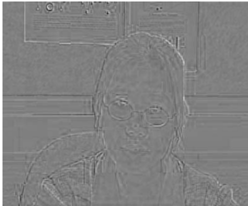
Figure 5.61 Residual to be encoded as enhancement layer
