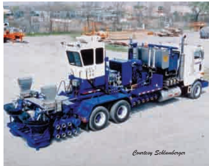
Fig. 5 —Modern fluid/proppant blender or proportioning unit.
