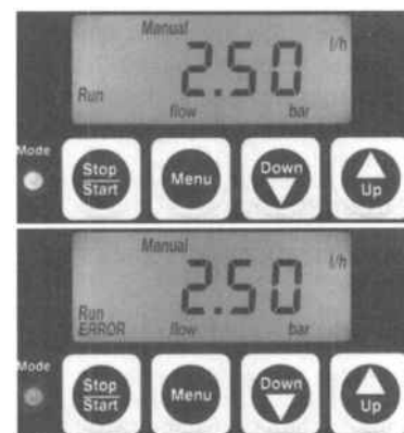
Figure 16.71 Display when pump is functioning correctly (upper). Display when there is a flow error (lower) Courtesy of Alldos Ltd
