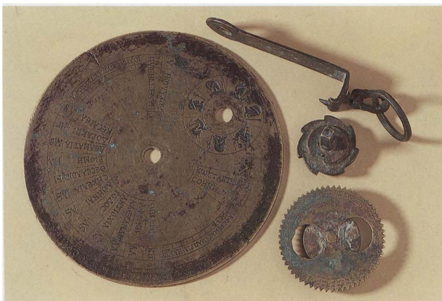
Figure 6 Fragments of Byzantine sundial-calendar, fifth or sixth century A.D. Brass gear wheel 52 mm diameter, with 59 teeth. (Collection Science Museum, London, inv. 1983-1393.)
