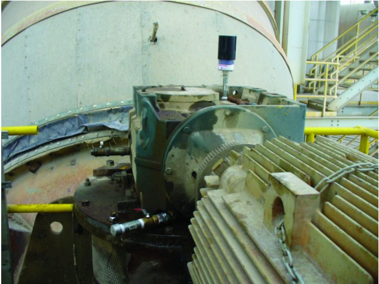
Fig. 1: The SEW Eurodrive gearbox, with Des-Case breather mounted on top.
