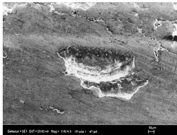
Fig. 11. SEM micrograph showing a typical pit caused by pitting on dedendum surfaces of the tooth.
