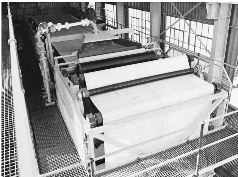
Figure 7.16. Delkor horizontal belt filter dewatering copper flotation concentrate (filter area 21 m 2 )
