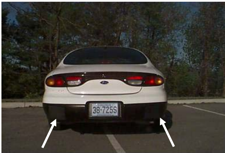
Figure 2.12. Rear Radar Units Embedded in Black Bumper.
