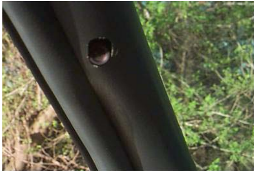
Figure 2.6. Driver's Face Camera Mounted in the A-pillar.
