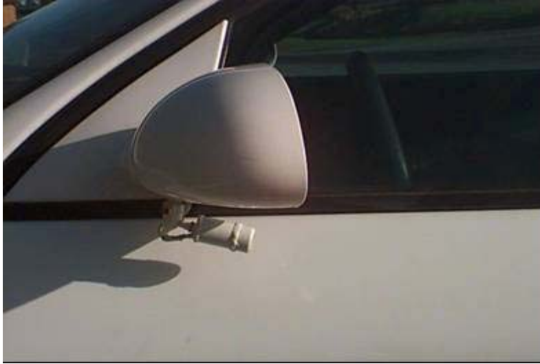
Figure 2.7. Camera Mounted Under the Side Mirror.
