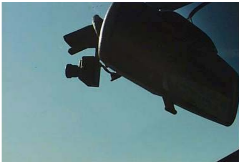
Figure 2.4. Forward View Video Camera Behind the Rearview Mirror.
