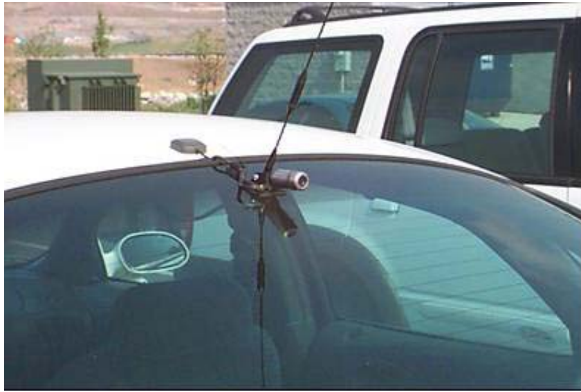
Figure 2.5. Rearview Video Camera above the Rear Window.
