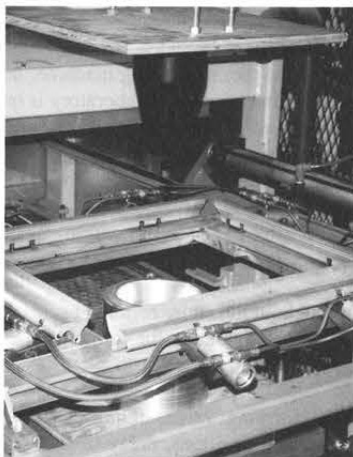
Figure A4.2 Close-up of the clamps, mold, and plug assist of the thermoforming machine
