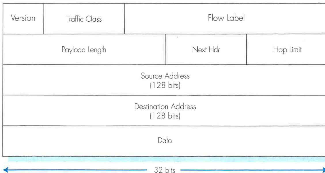
Figure 4.40 ♦ IPv6 packet format
