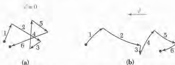
Fig. 1 Schematic path of an electron in a semiconductor. (a) Random thermal motion. (b) Combined motion due to random thermal motion and an applied electric field.
