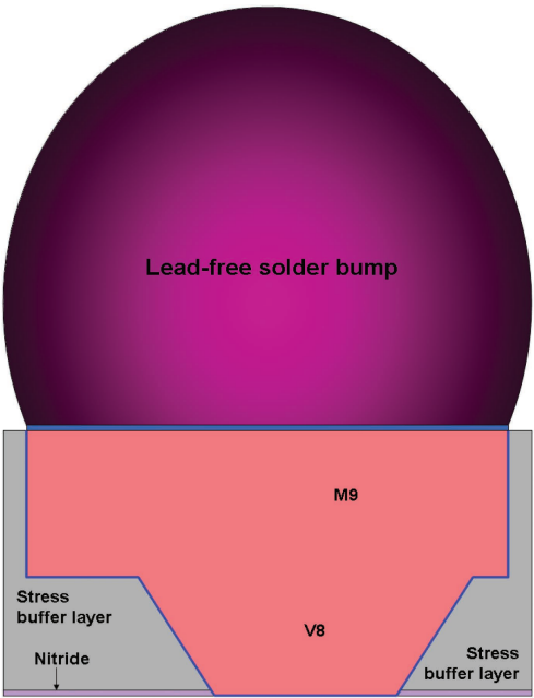
Figure 14.33 Lead-free solder bump formation.
