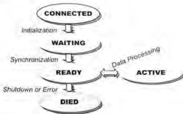
Fig. 2. Basic component states for module coordination
