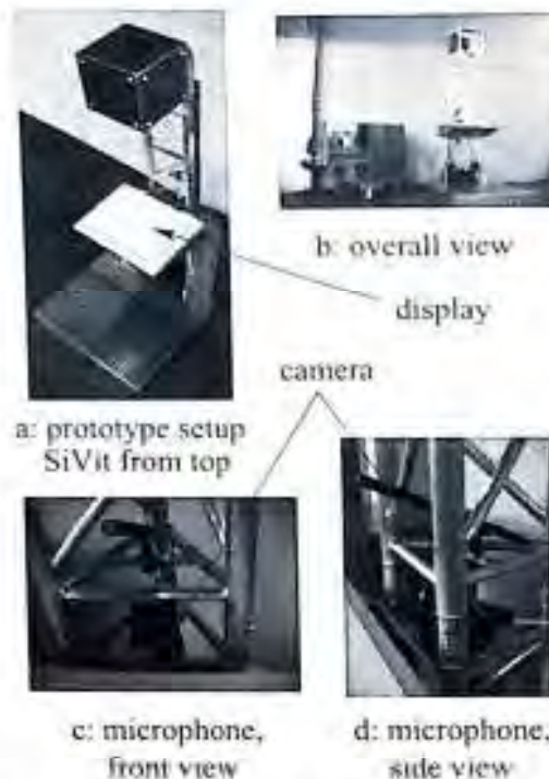
Fig. 1. SMARTKOM demonstration system. a prototype with integrated SiVit; b overall view with camera for facial expression analysis and microphones for speech analysis ( c,d )
