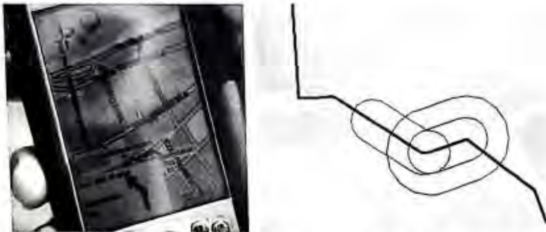
Fig. 4. Route segmentation and instructions. Left: SMARTKOM display with dynamically generated map, interface agent, and arrows indicating route direction. Right: Segmented route and trigger regions. Two regions around the active route indicate the valid and the egression region. The next route segment's valid region is also shown.
