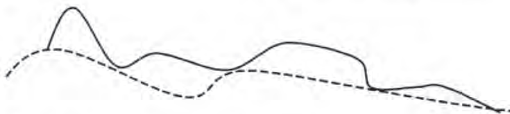
Figure 15.11 Composite contour obtained by low-pass filtering the impulses and boxes in the Fujisaki model of Figure 15.10.
