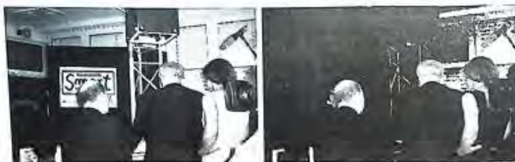
Fig. 2. Original image ( left ), result when skin-color segmentation is done ( right ). The image parts with blue and green color shades disappear, but white shades and natural colors stay
