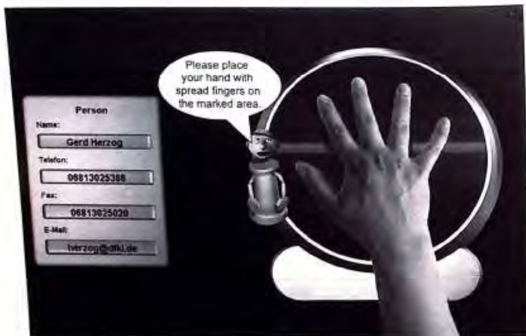
Fig. 6. Interactive biometric authentication by hand contour recognition
