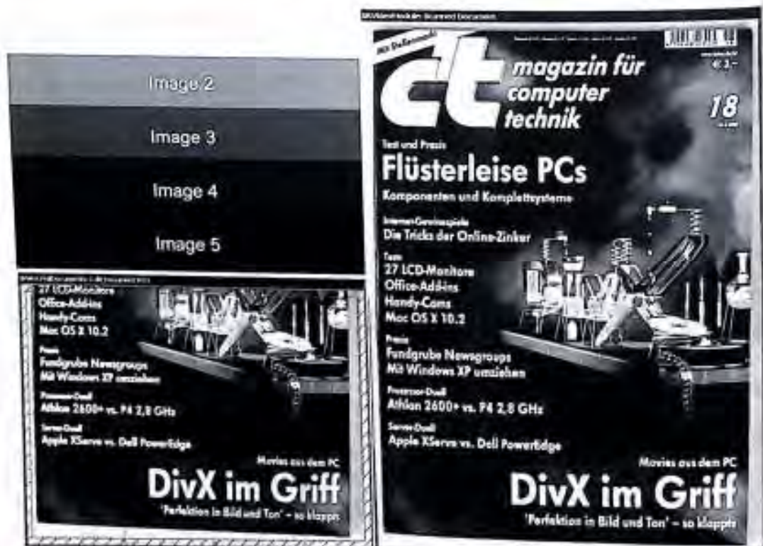
Fig. 7. Example of a (vertical) panoramic image creation. Recording of five overlapping images (scheme, top left) last (bottom) image (bottom left), resulting panoramic image (right)
