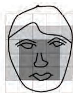
Fig. 2. A typical face used in knowledge-based top-down methods: Rules are coded based on human knowledge about the characteristics (e.g., intensity distribution and difference) of the facial regions [170].
