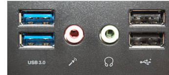
Two USB 3.0 Standard-A receptacles (left) and two USB 2.0 Standard-A receptacles (right) on a computer's front panel
