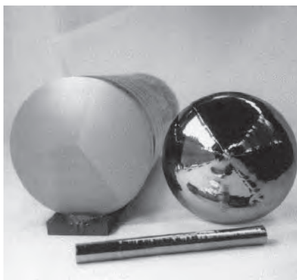
Figure 6.2 Tri-crystal seed (front), tri-crystal with cropped crown (left) and tri-crystal crown (right) with typical facets
