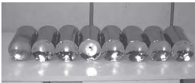
Figure 6.3 Tri-Si ingots ( 140 mm) from quasi-continuous pulling
