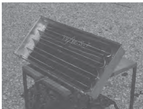
Figure 11.15 Static concentrator formed by an oil-filled CPC with bifacial cells
