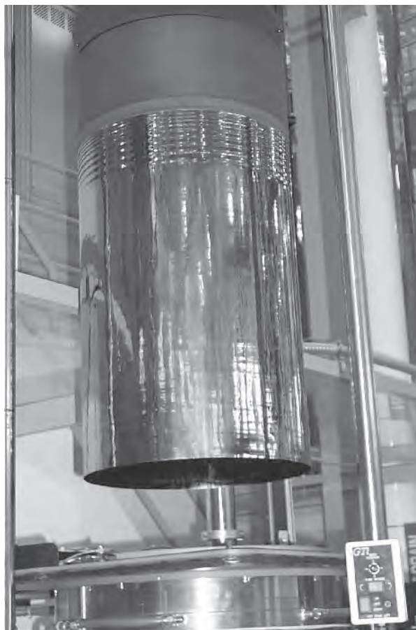
Figure 6.23 Experimental 50-cm-diameter EFG cylinder exiting from furnace
