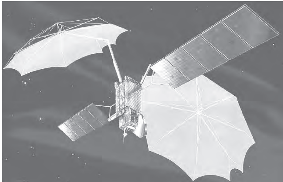
Figure 10.11 Rigid panel GaAs solar array (Picture courtesy of NASA). (The PV array is the two rectangular panels of five modules each)
