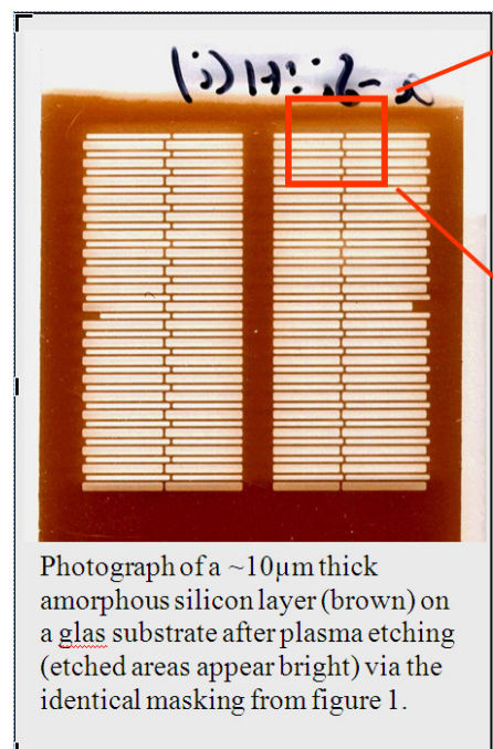
Figure 3: Structured a -Si:H layer after plasma etching through a flexible mask according to the novel method.
