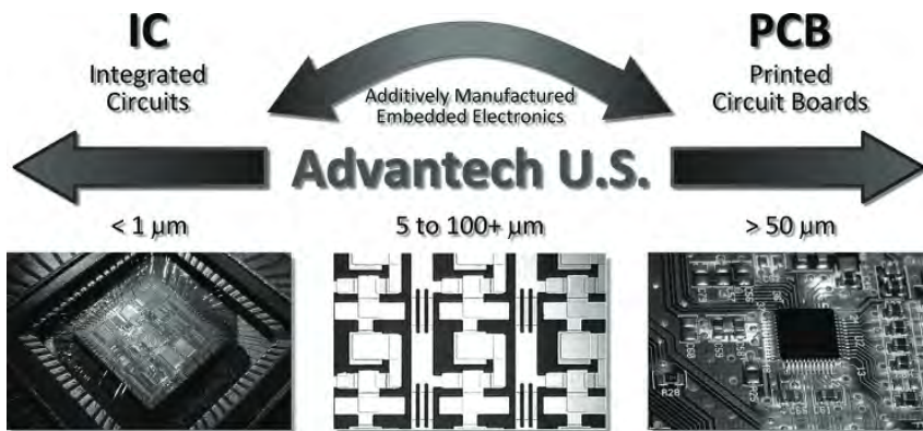
Figure 1. Bridging The Gap – Typical feature sizes in integrated circuit manufacturing, evaporation printing, and printed circuit board technology.
