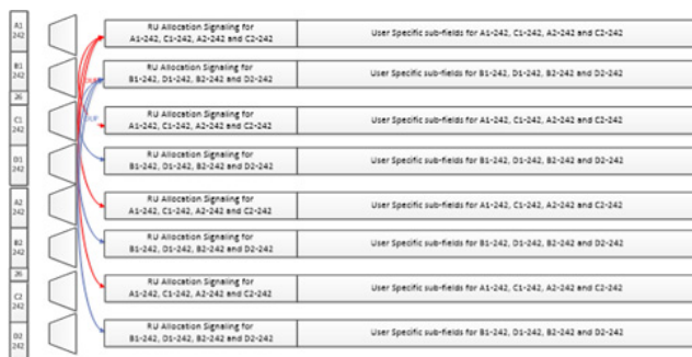
Figure 26-23—Default mapping of the two HE-SIG-B channels and their duplication in a 160 MHz PPDU
