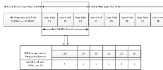
Figure 26-28—Illustration for the mapping of the 8-bit RU allocation subfield and the position of the user-field to the STA's assignment
