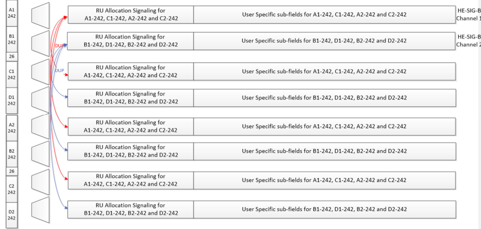
Figure 7 - Default mapping of the two HE-SIG-B channels for a 160 MHz HE PPDU
