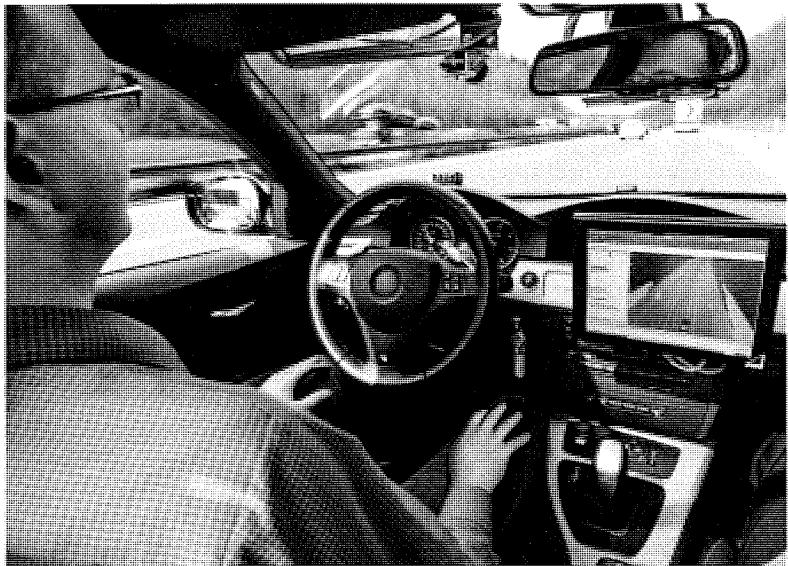
Fig. 7 A Bosch engineer supervising an automated vehicle test drive. The safety concept worked up for the test campaign was tested and approved by TÜV Süd. [2]
