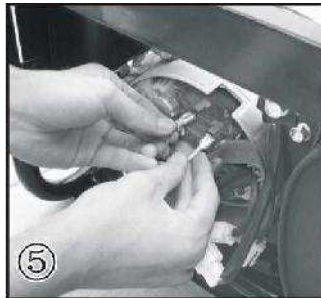
⑤ Insert and connect the 2 wires from the AVR, be sure to connect + and - correctly.
