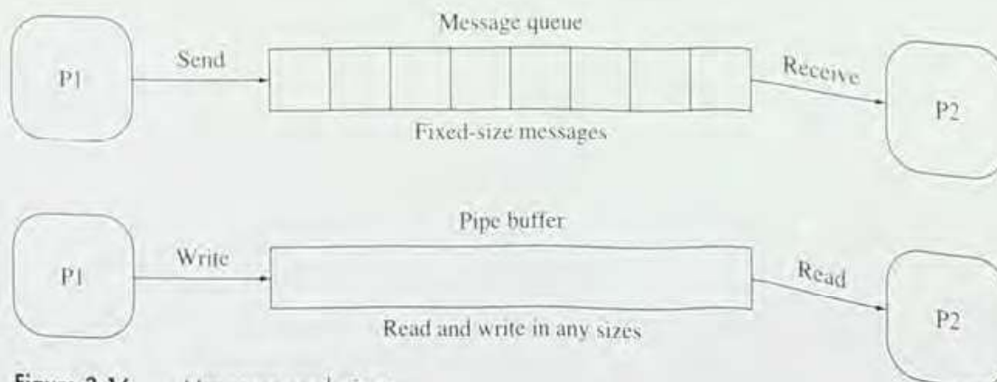
Figure 3.16 Messages and pipes
