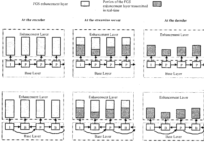
Fig. 1. Examples of the FGS scalability structure at the encoder (left), streaming server (center), and decoder (right) for a typical unicast Internet streaming application. The top and bottom rows of the figure represent base-layers without and with bidirectional ( B ) frames, respectively.
