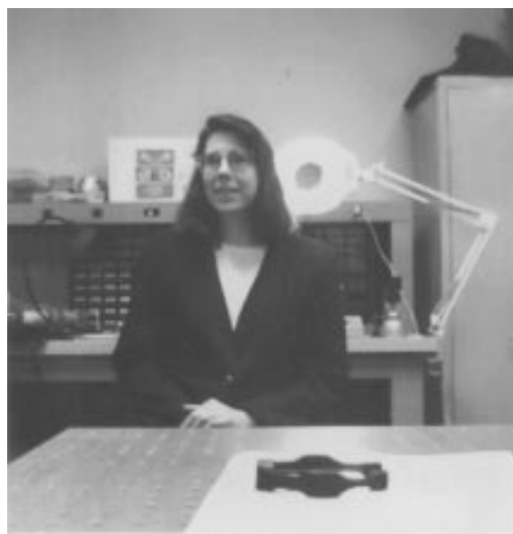
Fig. 10. Unprocessed image taken from a Photobit 256 \times 256 element sensor with on-chip ADC operating at 30 frame/s. Note no blooming from light and lack of other artifacts.
