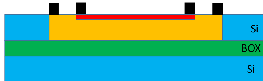
4. Etch microstructure holes
