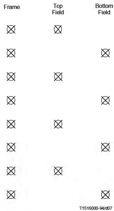
Figure 6-6 – Vertical positions of samples with 4:2:2 and 4:4:4 data
