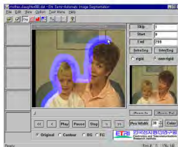
Figure F.11 — A graphical user interface for supporting intra-frame segmentation
