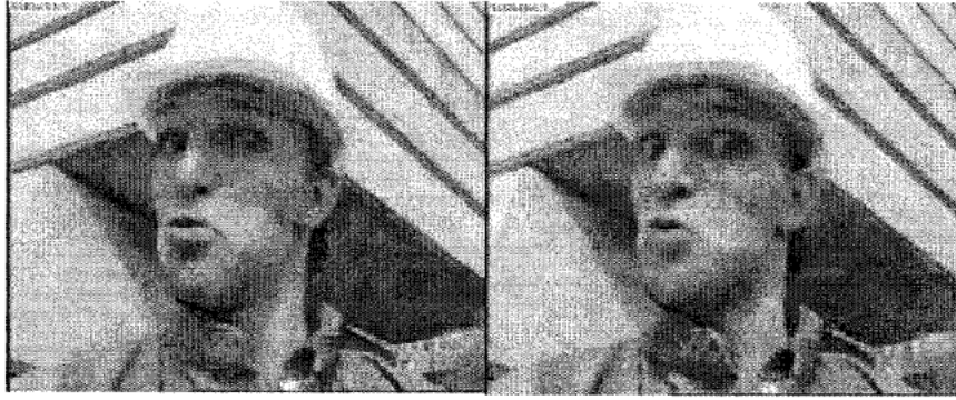
Fig. 12. Impact of employing frequency weighting on an FGS coded sequence. The left image is without frequency weighting while the right image is achieved by emphasizing low DCT frequencies.
